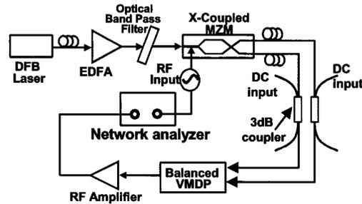
Fig. 4. Setup for measuring the nonlinearity of the distributed balanced receiver.
