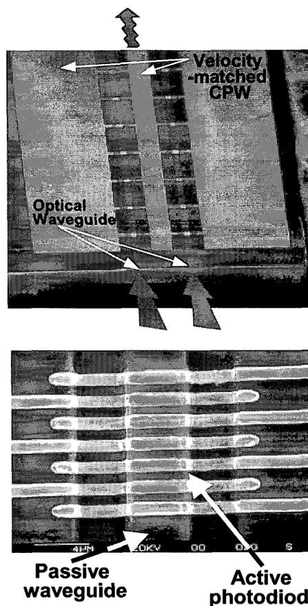
Fig. 1. (Top) SEM micrograph of the distributed balanced receiver. MSM photodiodes are distributed along the optical waveguide. (Bottom) Close-up view of a MSM photodiode on top of a multimode waveguide.
