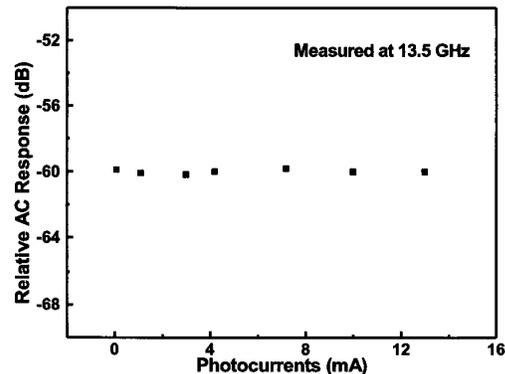
Fig. 5. Measured AC response of the balanced receiver at different photocurrent level. The response is linear at the photocurrent range within the experimental error of 0.5 dB.
