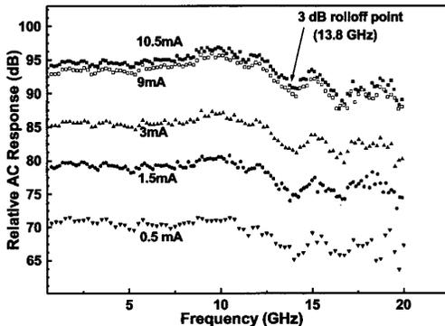
Fig. 6. Measured frequency response of the distributed balanced receiver at various DC photocurrents.
