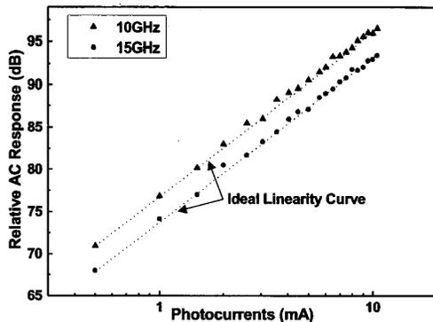
Fig. 3. Measured AC linearity of the balanced receiver at different photocurrents. The dotted line shows the ideal linearity curves.
