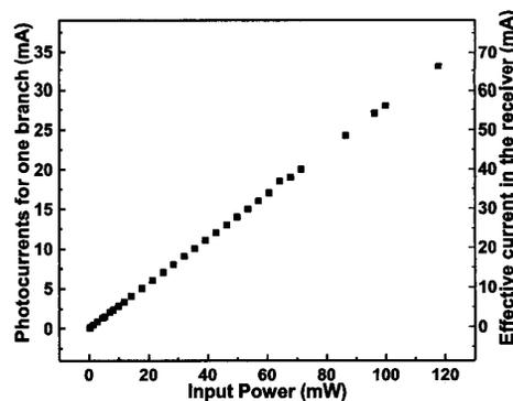
Fig. 2. DC photocurrent vs input optical power. The DC photocurrent remains linear up to  $33\text{ mA}$ .
